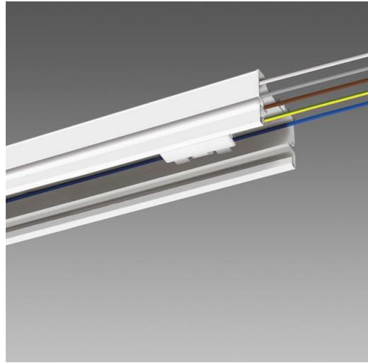
Supporting structure suitable for continuous light lines made with luminaires from the Techno System series or a combination of mixed luminaires. Quick and easy wall, ceiling or suspended mounting with the wide range of accessories. The track is supplied as standard with 5-pole, 7-pole (for EMergency and DIMMerable DALI versions) and 11-pole electrification, equipped with quick-connect terminal blocks.
