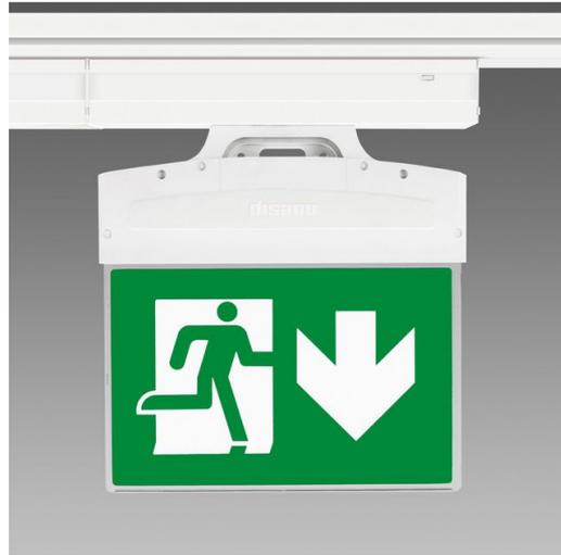
Techno System is designed to allow the installation of Safety Flag, through the appropriate unit. It is an emergency LED luminaire available in two versions: 1h life (recharge in 12h), 3h life (recharge 24h). In this case, too, mounting to the supporting channel is done in a practical way by means of the snap-on coupling system and is secured via a mechanical safety lock. This makes it possible to have general and safety lighting in one system.
