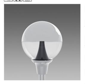
Globo: in polycarbonate, shatterproof and V2 self-extinguishing, UV stablised, anti-yellowing. Excellent transparency for good light transmission. Upper part painted to comply with light pollution regulations.
