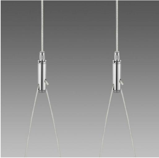
suspension complete with cable in steel with diam. 1.5 mm and length 0.5 m, including millimetric adjustment device. Max load: 20 Kg.
