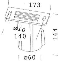
in die-cast aluminum. for installation on a 60 diameter pole in a two-lamp version.
