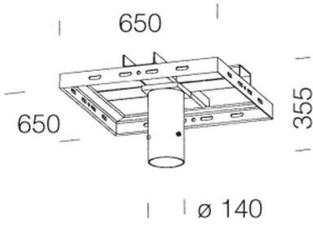
in die-cast aluminum. for installation on a 60 diameter pole in a two-lamp version.
